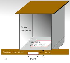
Detailed view for installation of Vacu Sweep: 170 x 60 mm (W x H)
