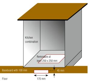
Detailed view for installation of dustpan: 170 x 45 mm (W x H)
